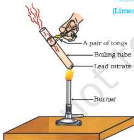
Figure 1.5 Heating of lead nitrate and emission of nitrogen dioxide
